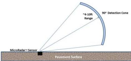
Like the M100 magnetometer wireless vehicle detector the M100BR bicycle radar sensor is small in size being only 74mm x 74mm x 58mm deep and is quickly and easily installed in the carriageway surface.
