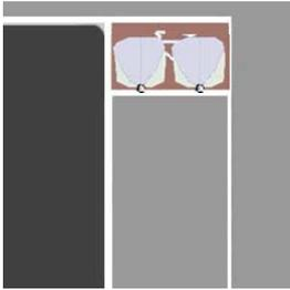
Secondly: two M100BR sensors are installed and OR'd together to detect bicycles arriving and stationary within the Advance Stop Line. The traffic signal controller would be configured to only take account of the detection input from the sensors during the red signal phase. Any other vehicle encroaching the Advance Stop Line during this red phase would not give a bicycle detect output.
