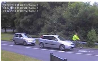
Using our own video verification software that overlays time stamped output information from the systems M120 interface contact closure card in the traffic signal controller onto a video of the location verification of the accuracy of the detector can be established.
