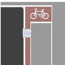
Firstly: the M100BR sensor is installed to detect bicycles within a cycle approach lane with its detection zone facing the kerb. In this configuration other vehicles passing in the main approach lane will not be detected. It should be noted that even if another vehicle enters the cycle lane the detector will differentiate between this and a bicycle and will not give a bicycle detect output.
