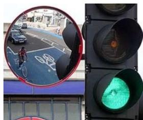
Trixi mirrors have been deployed at many junctions to enable HGV drivers to see more clearly any cyclists that would otherwise be in their blind spots. The Department for Transport have made it easier for a Local Authority to deploy such mirrors by removing the need to apply for permission each time.
